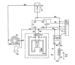
Ko: Power switch KM: AC contactor HA: Buzzer X1: Terminal FU: Fuse (25A) SJ: Thermostat SA: Sensitive switch CH1 CH2: Electrical heat tube KJ: Timer
